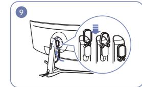
Hang the HOLDER-CABLE in the direction as shown in the figure.
