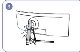
Push the COVER STAND BODY REAR in the direction as shown in the figure.
