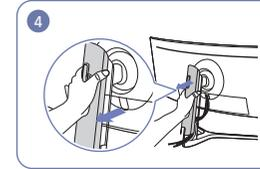
Remove the COVER STAND BODY REAR by pulling it in the direction as shown in the figure.
