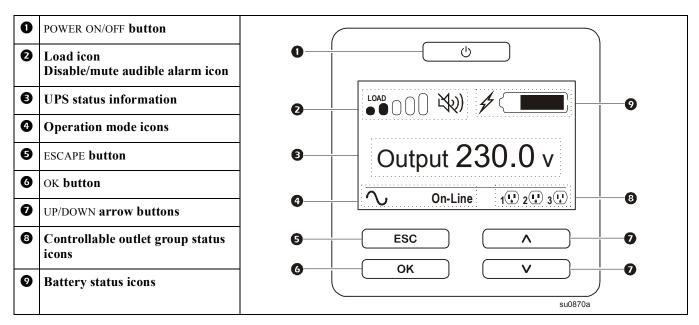
After RBCs are installed, the LCD shows a message to confirm if the installed RBCs are new. Select the correct option.
